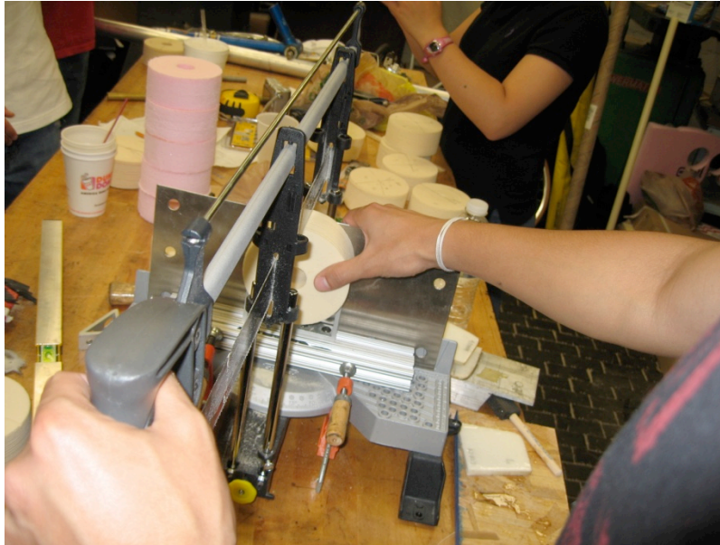
Figure 30: A hand saw was used to cut the discs at the proper angles
