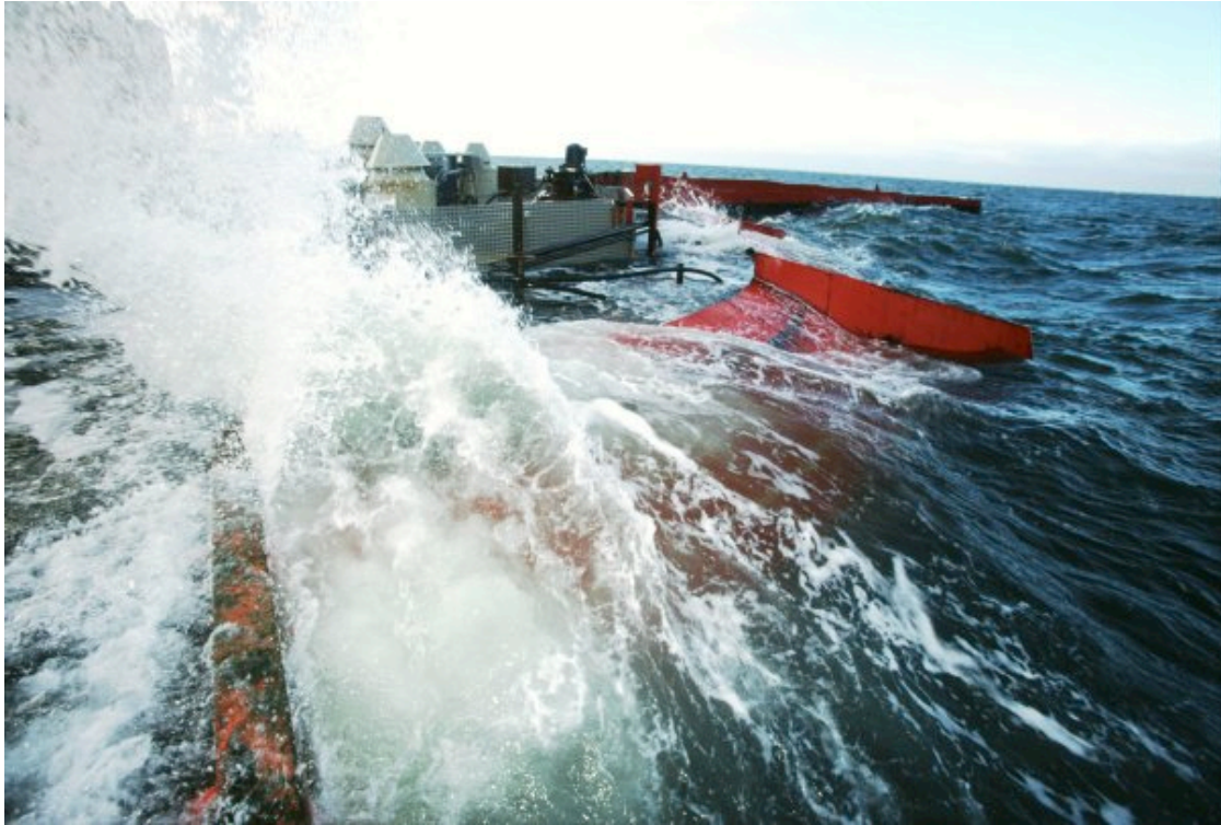
Figure 17: The WaveDragon overtopping device captures water in a reservoir as waves pass over the device (wavedragon.co.uk)
