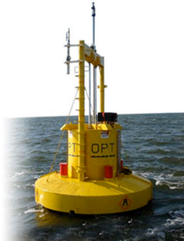
Figure 11: The Ocean Power Technologies PowerBuoy installed off the coast of Oregon (OPT, 2011)
